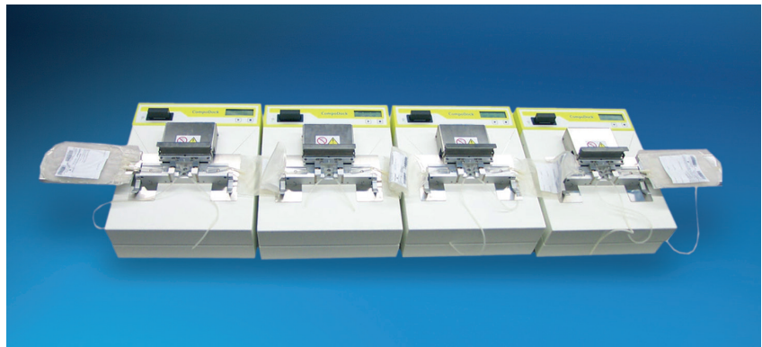
Highly efficient pooling by "chain" method: Docking of a pool of four buffy coats and one plasma in less than 1:20 minute. Ask for our promotion film.
